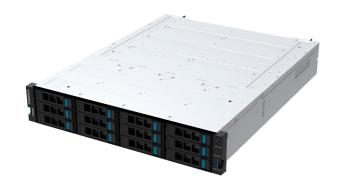
SD4100 is an economical 2U 12 drive bay enterprise-class SAS-4storage expansion platform with redundant architecture for greater data availability. It offers flexible, easy deployment, ideal for both small businesses and large enterprises that require a high level of efficiency and performance.
