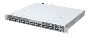
ES1000 provides 24x or 48x 1000Base-T and 4x 25GbE SFP28 ports in support of enterprise access, edge and data center management applications. The platform includes high-reliability features such as redundant fixed fans and hot swappable power supplies. ES1000 is available in both forward and reverse airflow configurations with optional 90W per port PoE++ support.
