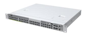
ES1050 includes high-reliability features such as redundant fixed fans and hot swappable power supplies. The platform is available in both forward and reverse airflow configurations with optional 90W per port PoE++ support.
